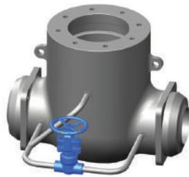
There is an additional connection between centre cavity and upstream for cavity relief. The gate valve is unidirectional.
