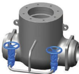
The arrangement consists of a connection between the centre cavity and a bypass pipe, with one valve each on the upstream and downstream of the bypass pipe. Based on the flow direction, one valve can act as bypass valve and the other, as a pressure equalizing valve. The gate valve is thus bidirectional.
