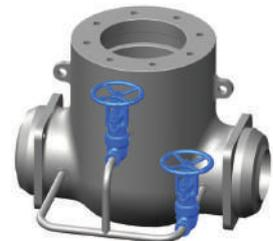
In this arrangement, the centre cavity is connected to a bypass pipe. Globe valves are provided on the downstream side and the connection between centre cavity and bypass. Entrapped fluid is relieved using the centre cavity valve. The gate valve is unidirectional.
